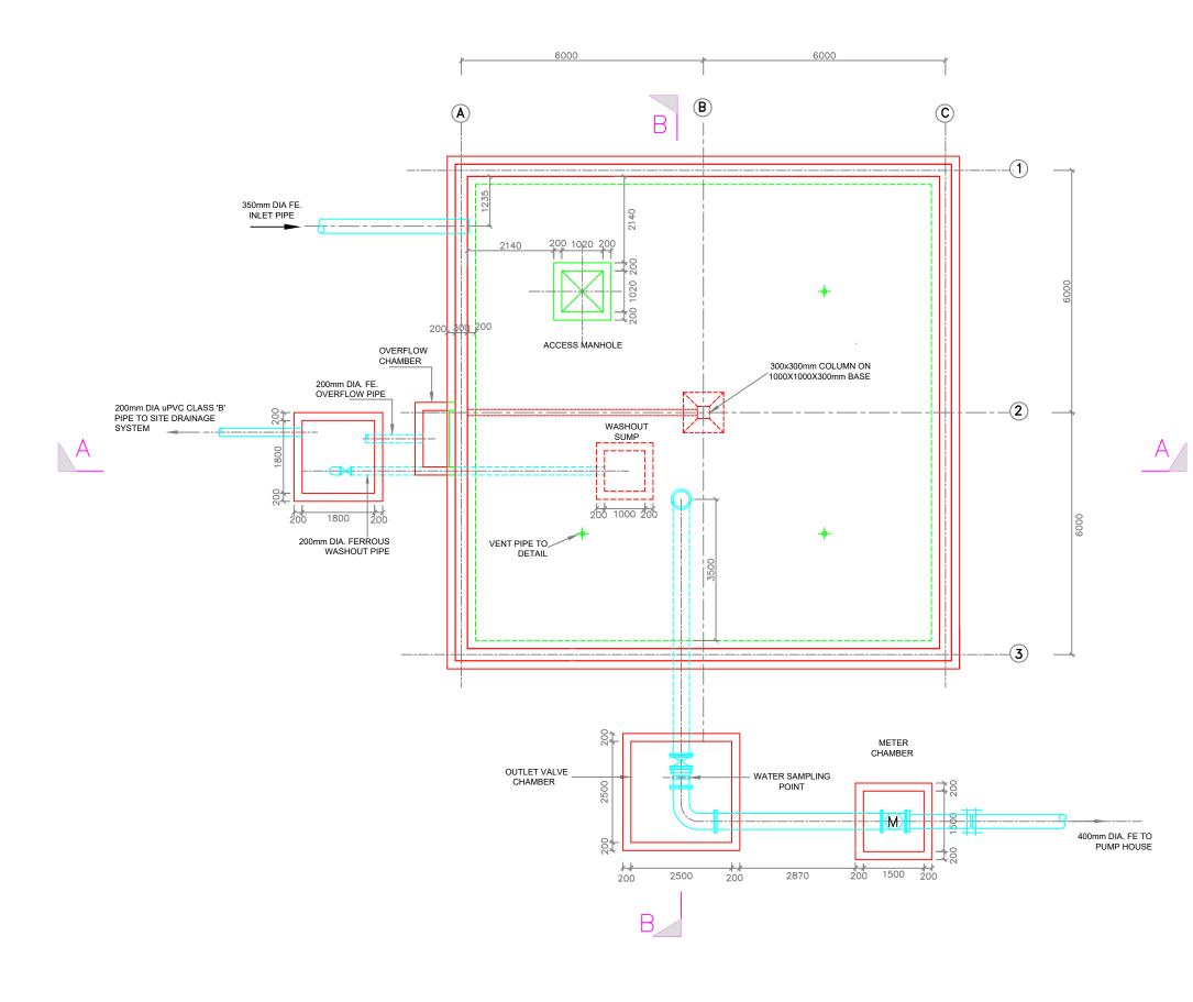
TREATED WATER TANK (500m<sup>3</sup>) ROOF SLAB PLAN
