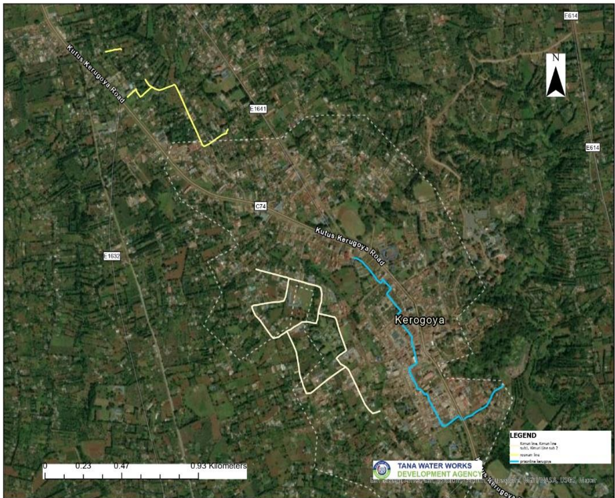
Figure 3 : Kerugoya Town Proposed Sewer Lines
